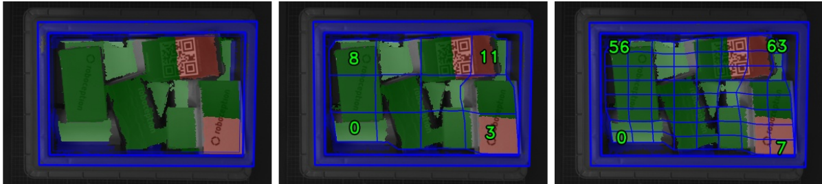
Fig. 6.5: Visualizations of the load carrier filling level: overall filling level without grid (left), 4x3 grid (center), 8x8 grid (right). The load carrier content is shown in a green gradient from white (on the load carrier floor) to dark green. The overfilled regions are visualized in red. Numbers indicate cell IDs.
