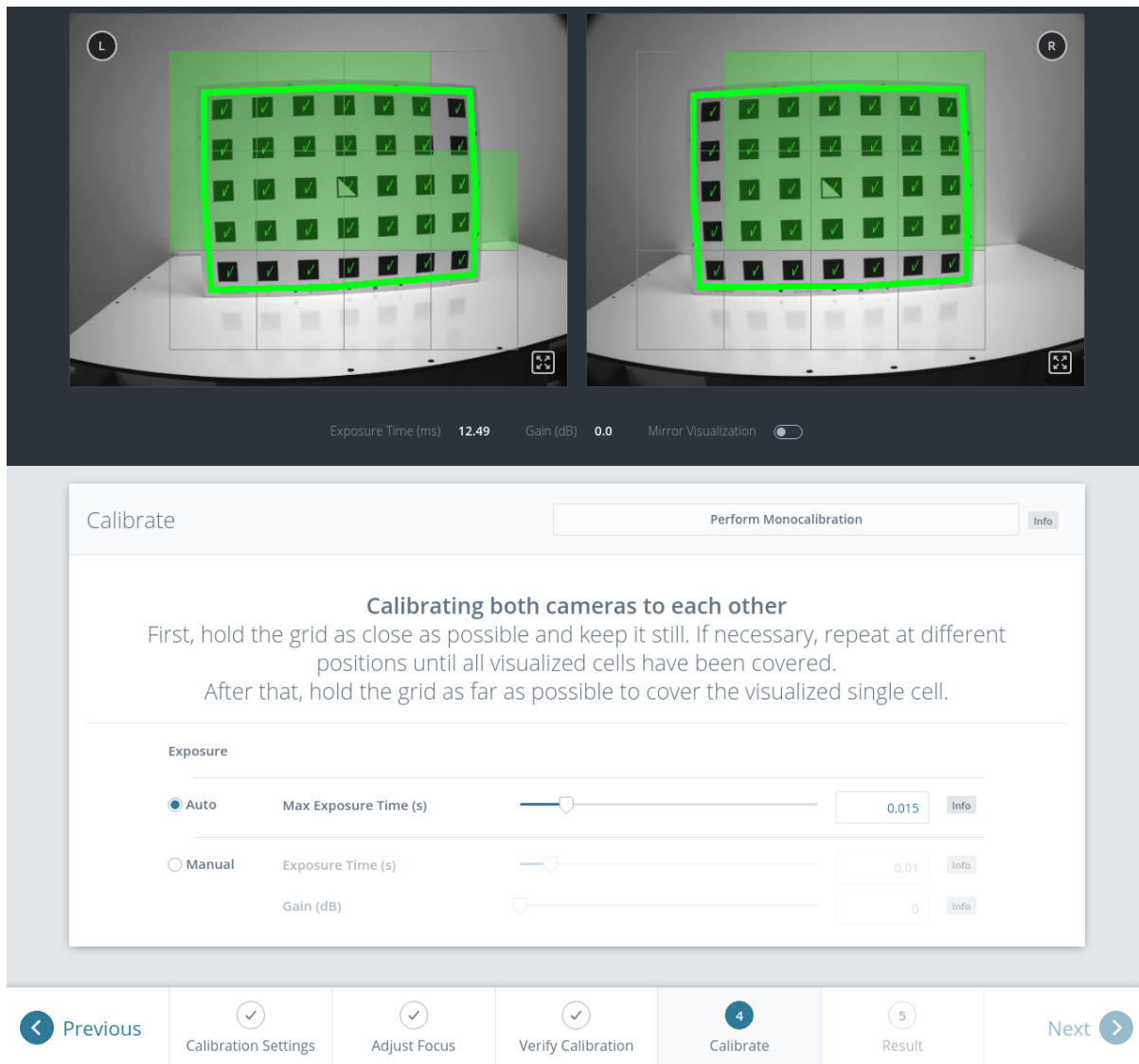
Fig. 6.31: Stereo calibration: Hold the grid as close as possible to fill all visualized cells
