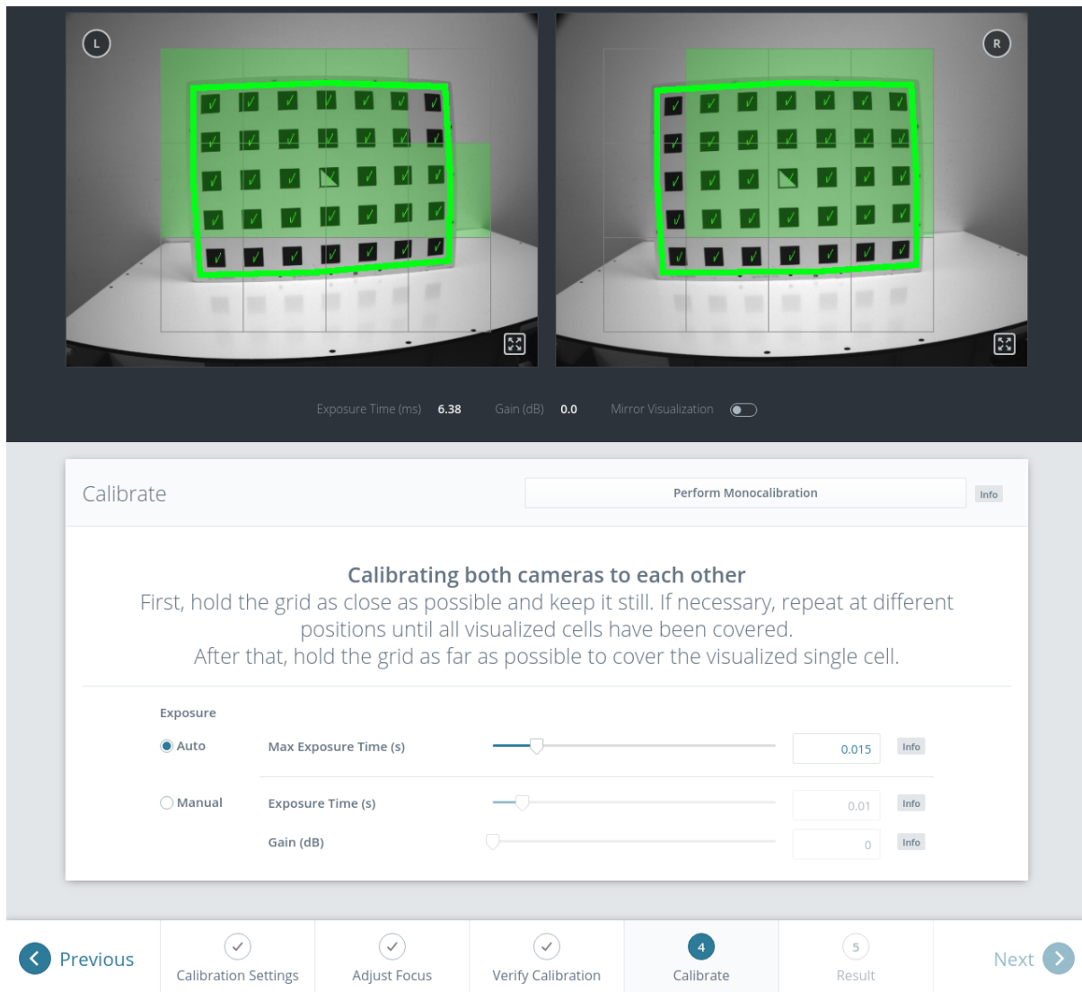
Fig. 6.32: Stereo calibration: Hold the grid as close as possible to fill all visualized cells
