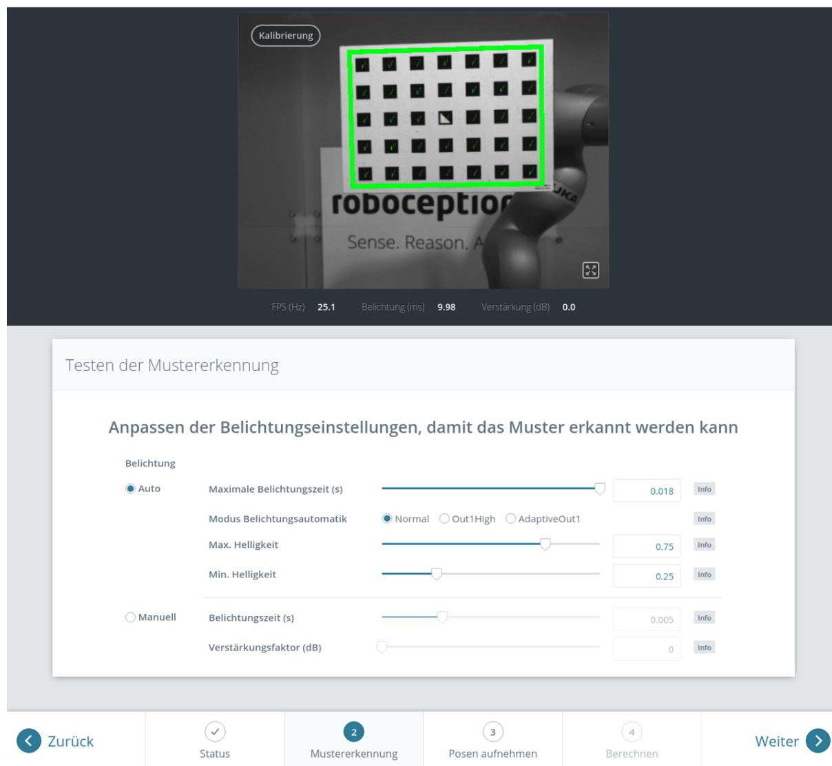
The screenshot displays the 'Kalibrierung' (Calibration) interface. At the top, a video feed shows a 5x5 grid of black markers on a white background, highlighted with a green border. Below the video, the following parameters are shown: FPS (Hz) 25.1, Belichtung (ms) 9.98, and Verstärkung (dB) 0.0.
