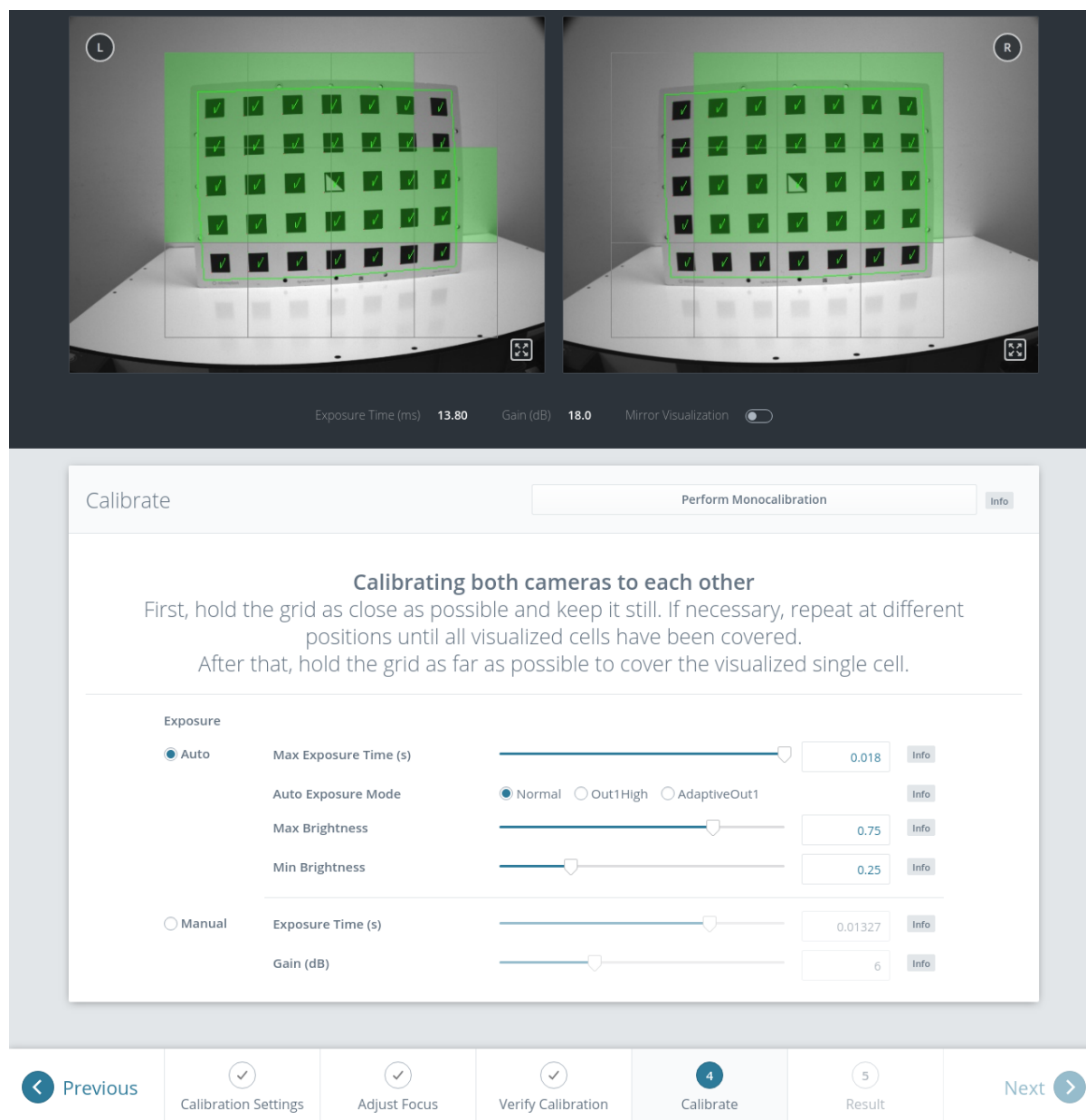
Fig. 6.33: Stereo calibration: Hold the grid as close as possible to fill all visualized cells
