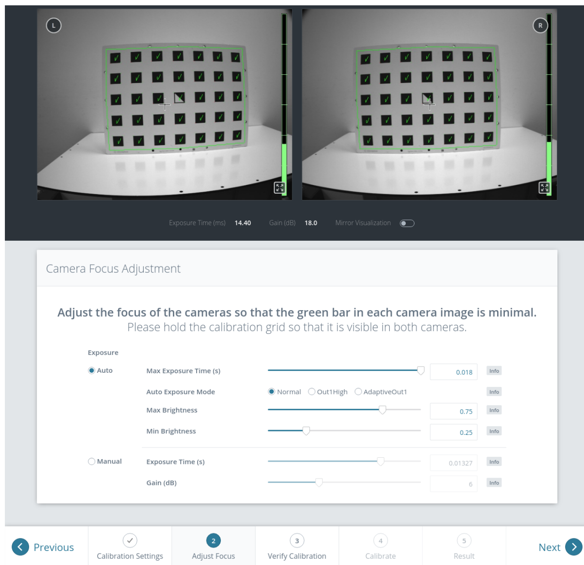
Fig. 6.30: Adjust the focus of each camera
