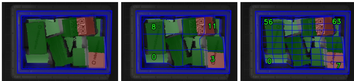
Fig. 5.8: Visualizations of the load carrier filling level: overall filling level without grid (left), 4x3 grid (center), 8x8 grid (right). The load carrier content is shown in a green gradient from white (on the load carrier floor) to dark green. The overfilled regions are visualized in red. Numbers indicate cell IDs.
